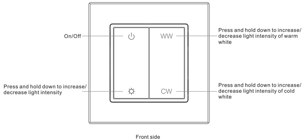
The remote control can be fixed on the wall with 3M glue or screw.
