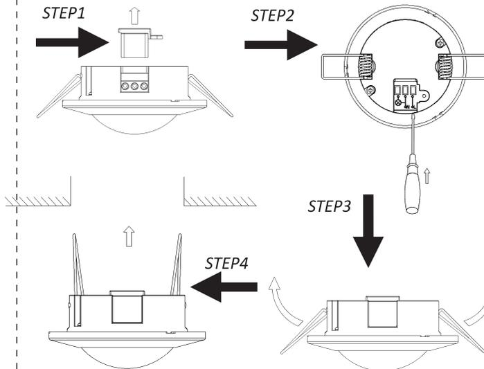
1. Turn off the main power supply and open the transparent plastic cover at the bottom of the sensor.
