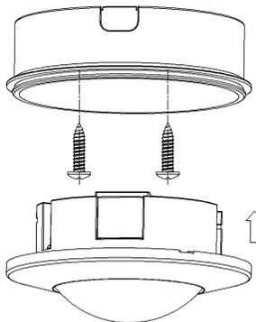
1. Turn off the main power supply and open the transparent plastic cover at the bottom of the sensor.
