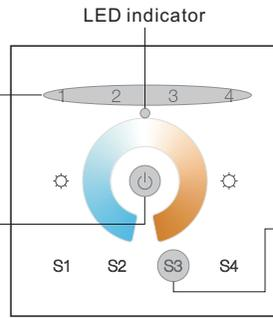
**Step 4:** Short press twice to enable the remote (target node) to find and unbind initiator. LED indicator flashes 4 times for successful unbinding or twice if unbinding fails.
