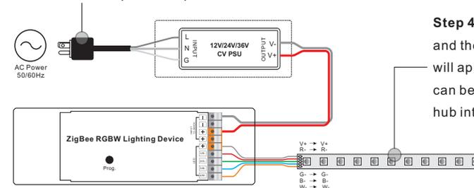
**Step 4:** Connected light will blink 5 times and then stay solid on, then the device will appear in your controller's menu and can be controlled through controller or hub interface.
