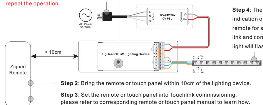
**Step 4:** There shall be indication on the remote for successful link and connected light will flash twice.
